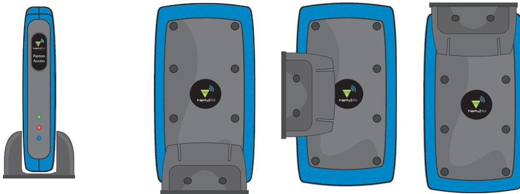
The antenna resides in the top of the box (with LED's at the base). Placing the box upright in this manner usually provides the best result for desk mounting the bridge and placing the ACU cabinet upright ensures that antenna lies in the same plane, again likely to provide the best results.
